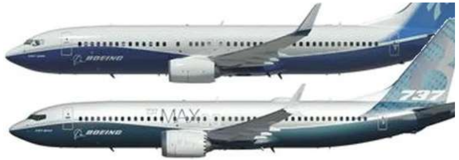
737 MAX vs NG Engine Placement and Size
